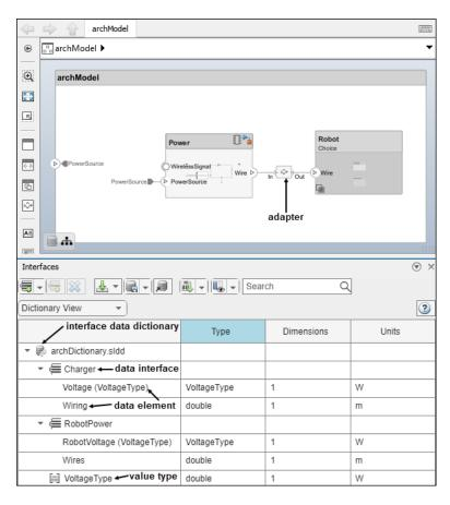
Manage owned interfaces local to a port using the Interface Editor in Port Interface View.
