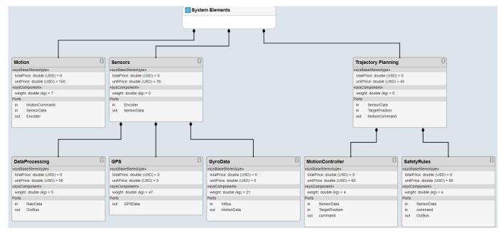
8 In the **Diagram** section of the toolstrip, click **Architecture Hierarchy** to display unique architecture types and their relationships using composition connections.
