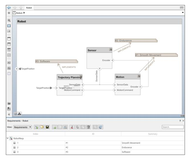
To enhance the traceability of requirements, link requirements to architectural components and ports. When you click a component in the Requirements Perspective, linked requirements are highlighted. Conversely, when you click a requirement, the linked components are shown. To directly create a link, drag a requirement onto a component or a port.
