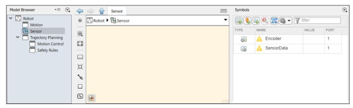
Select the **SensorData** output and view the interface in the **Property Inspector**. You can access this interface like a Simulink bus signal.
