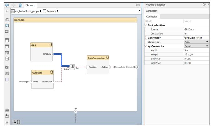
Finish defining metadata across the model for each element using desired property values. Pin the **Property Inspector** to the editor to keep the **Property Inspector** visible during this operation.
