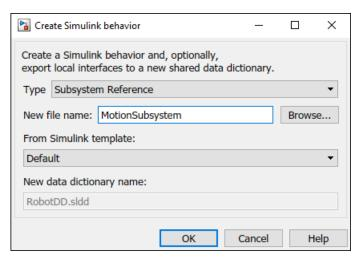
A new Simulink subsystem file with the provided name is created in the current folder. The root-level ports of the Simulink subsystem reflect the ports of the component. The component in the architecture model is linked to the Simulink subsystem. The component indicates that the component has a Simulink subsystem behavior.
