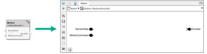
**4** To view the interfaces on the **SensorData** port converted into Simulink bus elements, double-click the port in Simulink.
