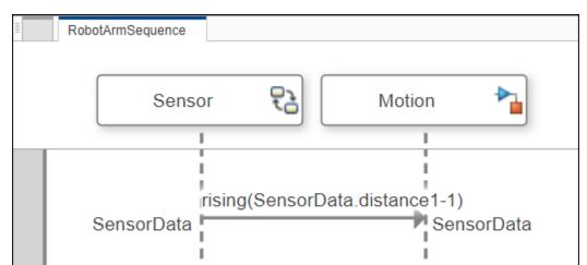
The signal name is a data element on a data interface. The message will be recognized at the zero-crossing event when the value of SensorData.distance1 rises to 1.
