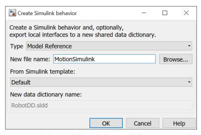
A new Simulink model file with the provided name is created in the current folder. The root-level ports of the Simulink model reflect the ports of the component. The component in the architecture model is linked to the Simulink model. The icon on the component indicates that the component has a Simulink behavior.
