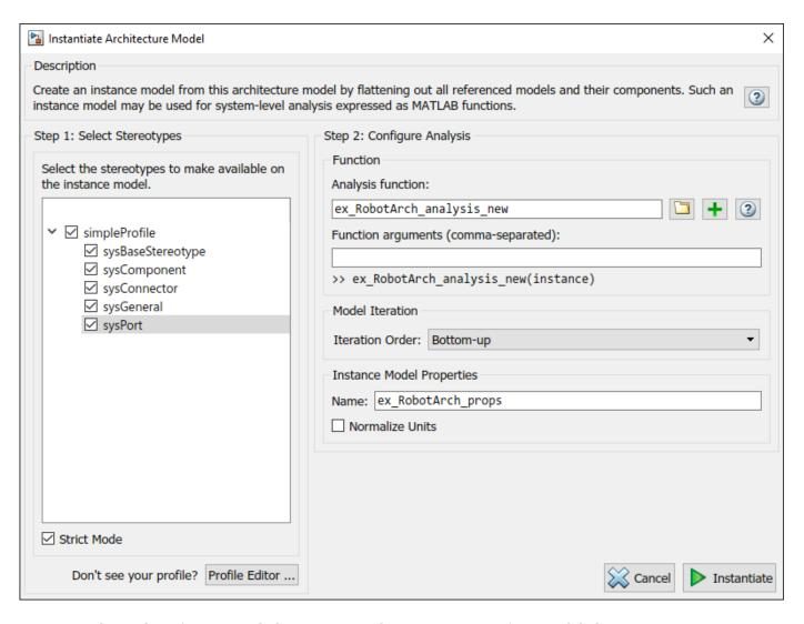
The analysis function includes constructs that get properties from model elements, given as a template. Modify this template to add the cost of individual elements and obtain total cost for their parent architecture. This function computes the cost for one model element as a total of its own cost and the cost of all of its child components. Copy and paste the function below into your analysis function.
